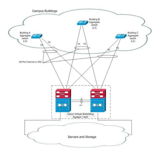
In the diagram, we have Campus building aggregate switches running L2 functionality linked to a Cisco VSS 1440 system acting as the Layer 3 core of the network (the VSS 1440 systems are effectively 2x Catalyst 6509 units configured as a single logical unit if you are not familiar with them). Each aggregate switch has a 1Gb link to each of the 6509 chassis,
